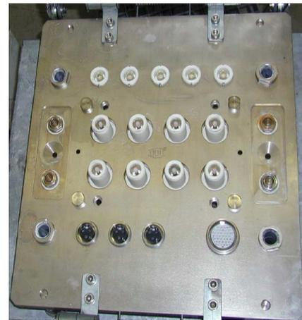
Figure 4: XFEL Power Supply Rack Docking Station for fast installation/replacement of entire rack
