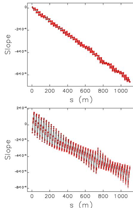
Figure 1: Betatron phase slope with rf frequency – top is horizontal plane, bottom is vertical plane.
