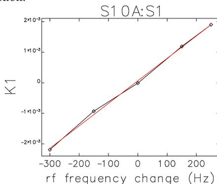
Figure 4: Results of the response matrix fit for the test sextupole and the linear fit (red line).
