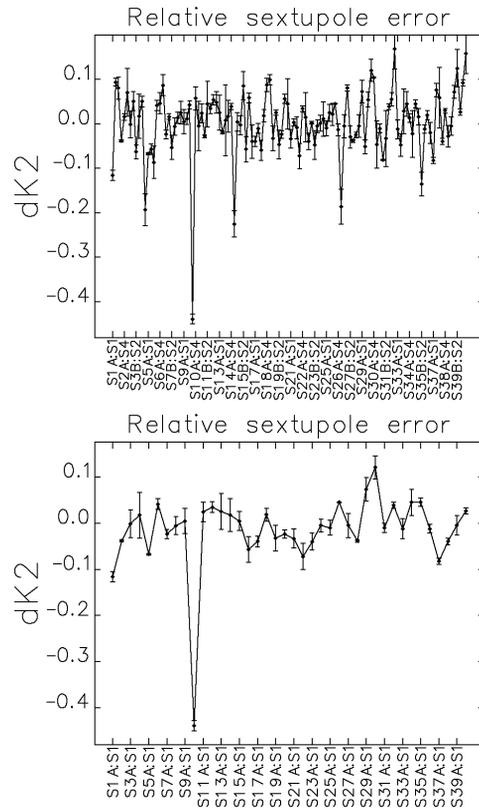
Figure 5: Measured corrections to sextupole *K2* values. Top plot – all sextupoles used in the response matrix fit, bottom plot – only the S1 sextupole family; the test sextupole clearly stands out.
