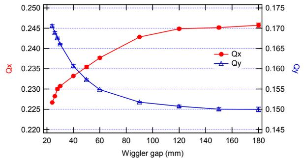
Figure 6: Measured tunes as a function of the wiggler full gap in the BBY6T mode.
