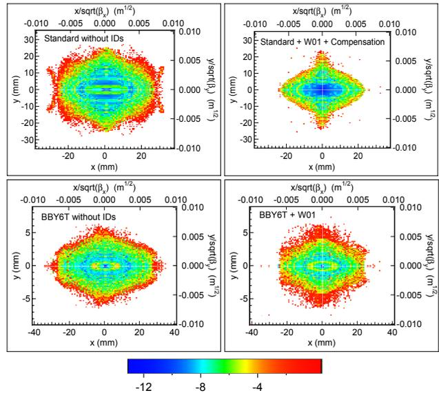
Figure 5: Dynamic aperture for the Standard (top row) and BBY6T (bottom row) modes. From left to right we have the lattice without IDs and with the 2.0 T wiggler with compensation in the Standard mode. The color code indicates the change in betatron tunes in a logarithmic scale.
