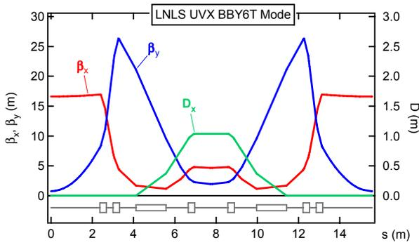
Figure 2: Twiss functions for the BBY6T mode.
