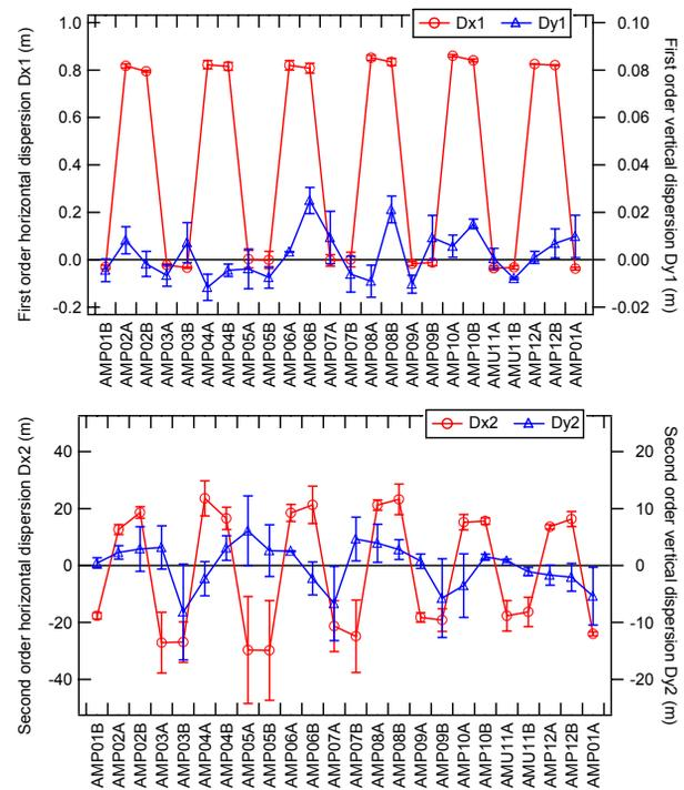
Figure 9: Measured first (top) and second (bottom) order dispersion function.
