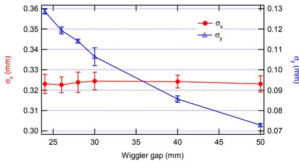
Figure 7: Measured beam-sizes as a function of the wiggler full gap in the BBY6T mode.
