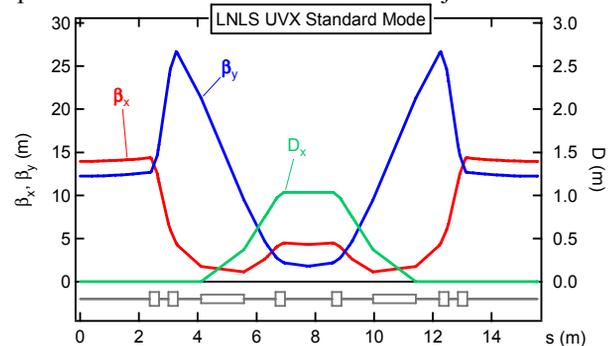
Figure 1: Twiss functions for LNLS UVX Standard mode.
