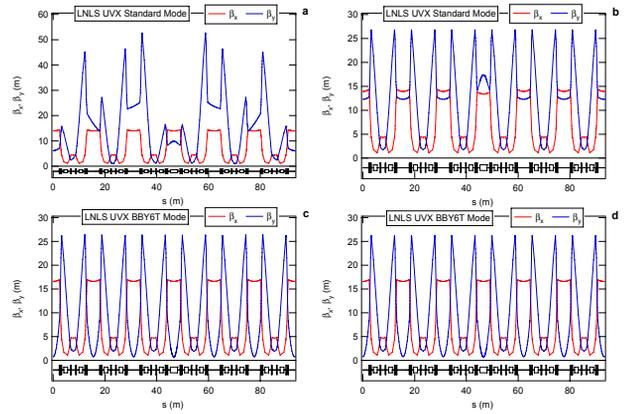
Figure 4: Linear optics perturbation caused by a 2.0 T multipole wiggler on the LNLS ring. (a) and (c) show respectively the Standard and BBY6T modes without compensation and (b) and (d) with compensation.
