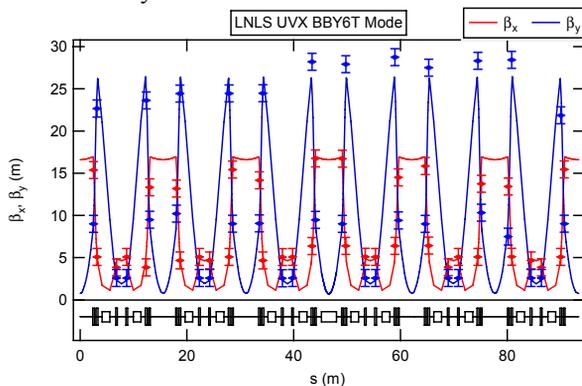
Figure 8: Measured (dots) and calculated (full curves) betatron functions in the BBY6T mode with the wiggler closed. The betatron functions were measured by changing quadrupole strengths.
