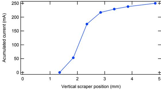
Figure 3: Saturation current at injection as a function of the vertical scraper position (half-gap height).
