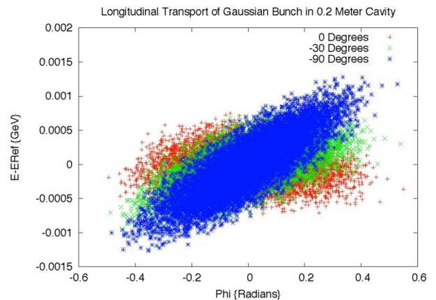
Figure 4. Longitudinal phase space distributions of 6D Gaussian bunch for different phases.
