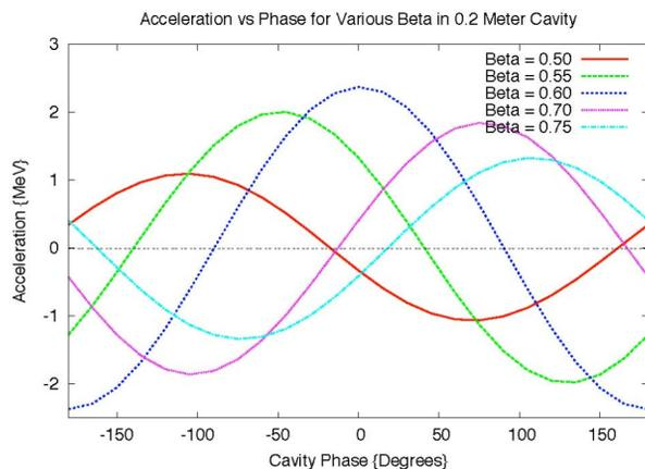
Figure 3. Energy gain versus relative phase for a cavity of length 0.2 m.
