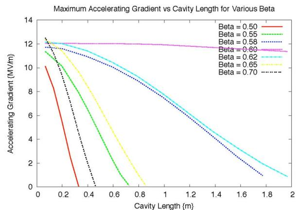
Figure 1. Maximum accelerating gradient versus cavity length for particles of different  $\beta$ .
