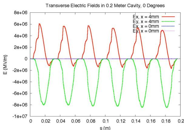
Figure 6. Vertical and horizontal electric fields seen by particle at  $\beta = 0.6$  and  $0^\circ$  phase for  $x = 0$  mm and for  $x = 4$  mm.
