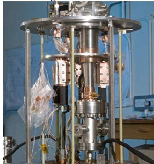
Figure 6: The cryostat turret.
