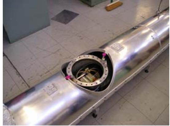
Figure 5: He vessel and magnets inside radiation shields.
