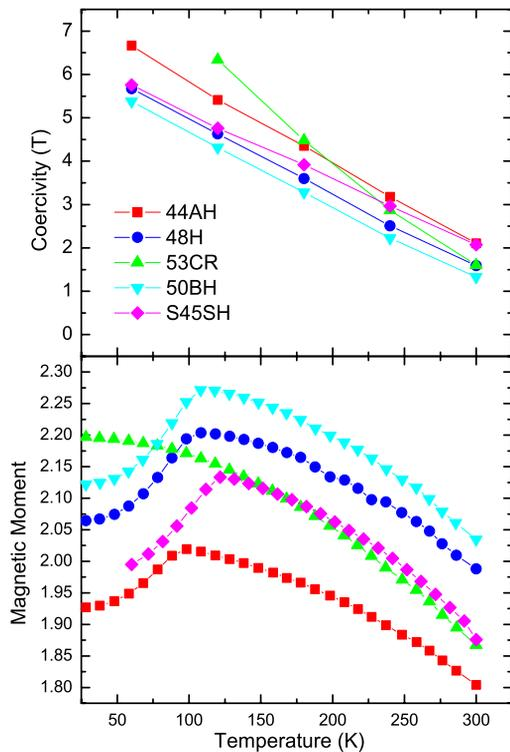
Figure 2: Temperature dependence of remanence for various kinds of PM material. All of the PM material have been supplied by Hitachi Metals. The prefix “NEOMAX” have been omitted from the material names for simplicity. Note that remanence is indicated by the magnetic moment of the PM sample.
