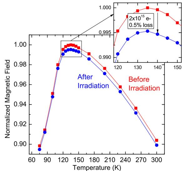
Figure 1: Temperature dependence of remanence of NEOMAX50BH before and after electron irradiation.
