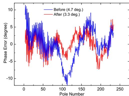
Figure 5: Example of the field correction by the differential adjuster applied to the CPMU for SLS at RT. Note that this is not the final status of the phase error.
