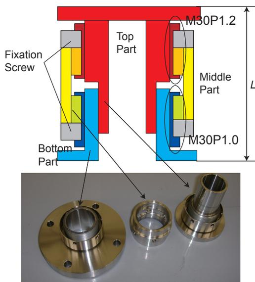
Figure 4: Differential adjuster for the adjustable outer shaft.
