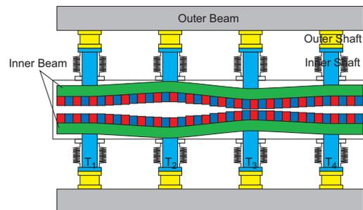
Figure 3: Gap variation induced by the temperature gradient.
