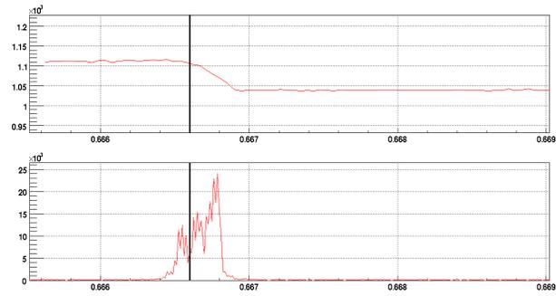
Figure 12: Total intensity decrease (upper plot) and particles loss rate (lower plot) during the resonance crossing. Tune change 0.6687→0.6653 for 1 s,  $I = 0.212 \rightarrow 0.214$
