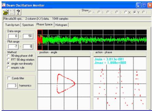
Figure 11: Measured phase trajectories close to the third-order resonance.
