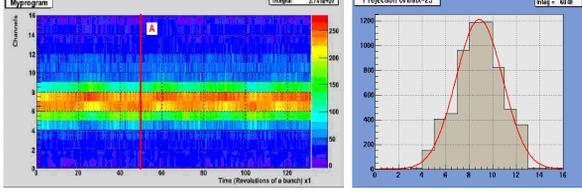
Figure 2: The vertical beam profile vs. revolution number (left plot). Colors indicate the beam intensity. Single shot vertical beam profile fitted by the Gauss function (right plot).
