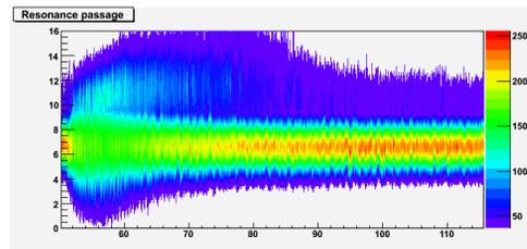
Figure 7: The same as in Fig.5 but the crossing time is 0.3 s. A beam blow-up and some evidence of the particles trapping are observed.
