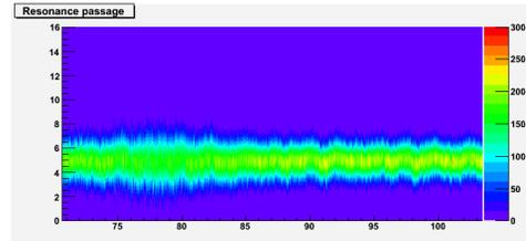
Figure 6: Tune range is  $Q_z = 0.6608 \pm 0.6717$ ; crossing time is 40 ms. For high rate neither beam size change nor particles capture is seen.
