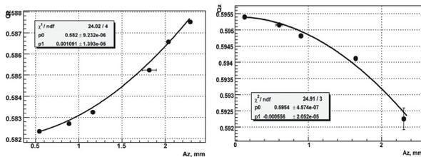
Figure 3: Vertical tune vs. amplitude for different currents in the octupoles. Polarity changing gives the tune shift term change from  $C_{zz} = 1 \times 10^{-3} \text{ mm}^{-2}$  to  $C_{zz} = -0.5 \times 10^{-3} \text{ mm}^{-2}$ .
