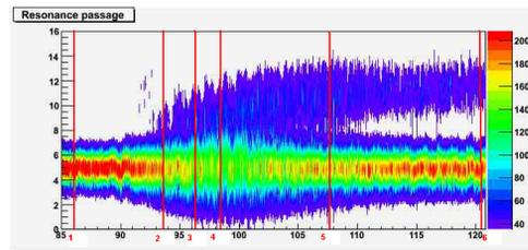
Figure 8: Time evolution of the vertical beam profile in the case of the particle trapping in the resonance island ( $\Delta t = 3$  s).
