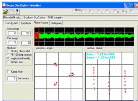
Figure 5: Measured trajectories inside the resonance island.
