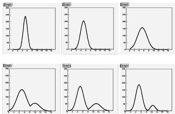
Figure 9: Transverse distribution of the beam profile (Gauss fit of the MAPMT 16 channels) corresponding to the different moments indicated by the red lines in Fig.8.
