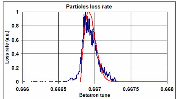
Figure 13: The vertical betatron tune change  $\Delta\nu_z = 0.6653 \rightarrow 0.6685$  for 1 s,  $I = 0.183 \rightarrow 0.181$
