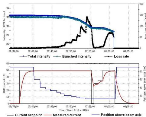
Figure 5: Long-range beam-beam experiment in RHIC with deuterons at store. The upper plot shows the total and bunched beam intensity (blue curves) and the calculated beam loss rate (black curve). The lower plot shows the set point for the wire current (black curve), the measured current (red curve), and the wire position above the beam pipe center (blue curve).
