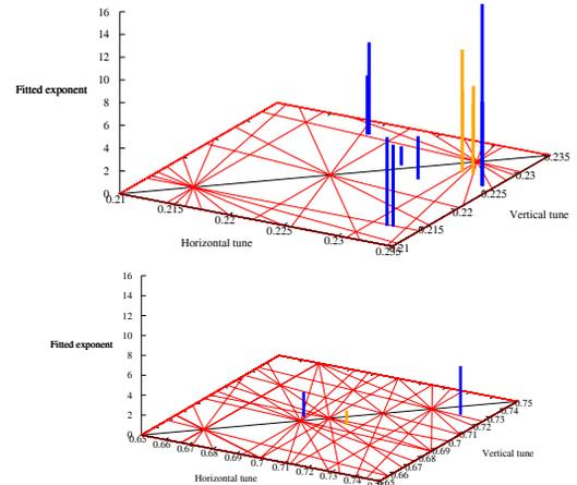
Figure 6: Fitted exponents  $p$  for long-range beam-beam experiments as a function of the ion tunes (top) and the proton tunes (bottom). The fitted exponents range from 1.7 to 16.
