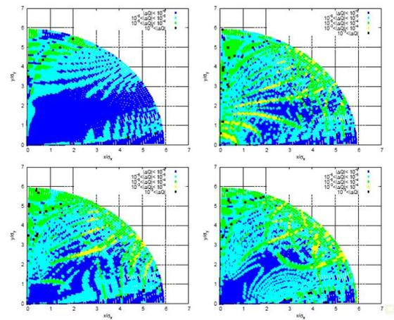
Figure 8: Tune diffusion without beam-beam interaction (top left), with beam-beam interaction (top right), with half (bottom left), and with full beam-beam compensation [32].
