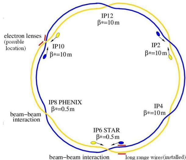
Figure 1: Beam-beam interactions in RHIC and locations of wires and electron lenses. The shown  $\beta^*$  values are for the polarized proton design configuration at 250 GeV, which has not been implemented yet.
