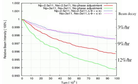
Figure 9: Beam lifetime simulations for increased bunch intensity and different phase advances between the IP and e-lens. Note that without compensation the beam-beam tune generated tune spread could not be accommodated for these bunch intensities.
