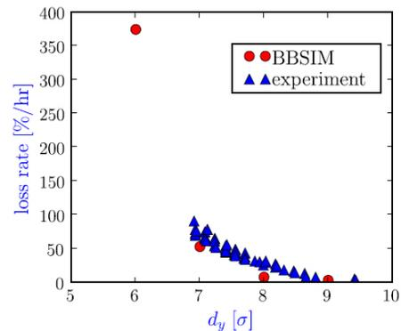
Figure 7: Comparison of measured and simulated beam loss rate as a function of distance between wire and beam. Experiment with gold beam at store, wire strength of 125 A m [24].
