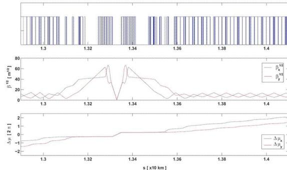
Figure 2: LHC IR lattice functions. At  $s = 13.433$  km, with approximately equal transverse  $\beta$ -functions, a long-range wire compensator or electron lens could be placed.
