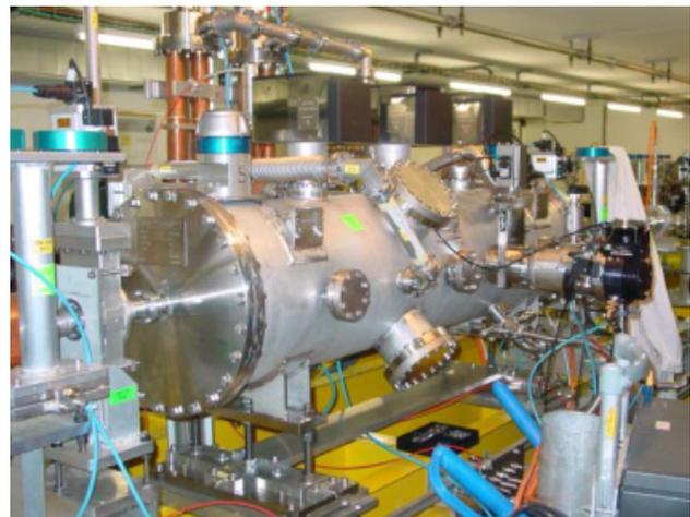
Figure 6: The PETS tank installed in the TBTS test area.
