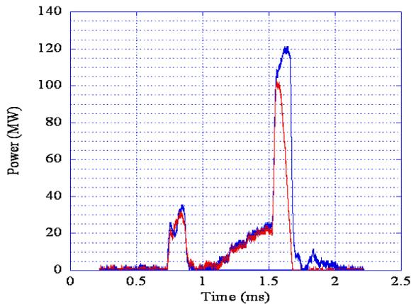
Figure 4: Typical transmitted RF pulse in ASTA (blue) and the pulse with breakdown event in the PETS (red).
