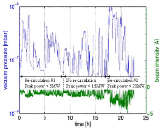
Figure 7: The vacuum and drive beam current history together with a brief summary of the system settings.
