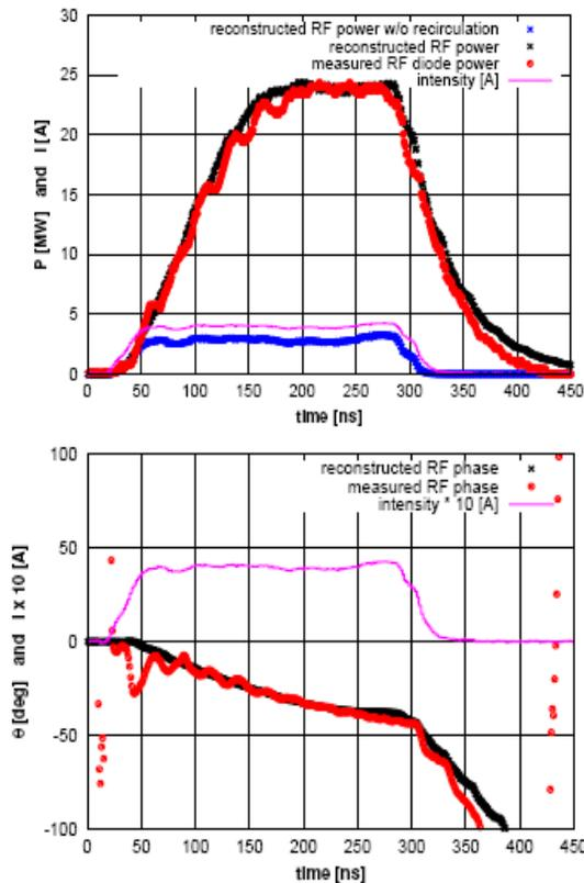
Figure 8: The measured (red) and reconstructed (black) RF power pulses (upper plot) and RF phases (low plot). The drive beam current (magenta) and expected power production without re-circulation (blue) are given for reference.
