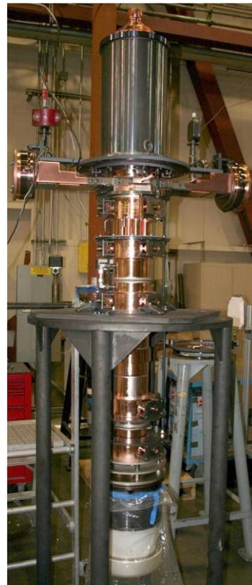
Figure 1: The vacuum envelope of the VKL-8301B prototype, serial number 002, being prepared for dress after bakeout.
