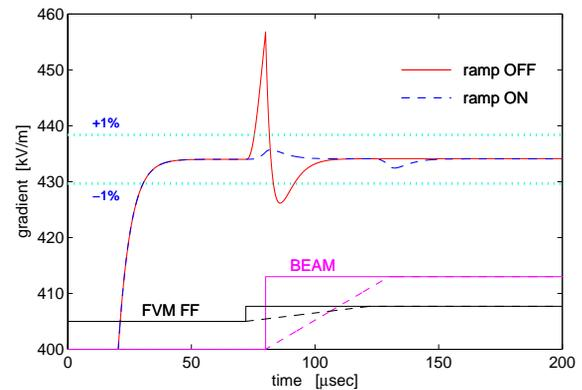
Figure 4: Beam compensation with FVM transient response for HINS cavity no. 6.
