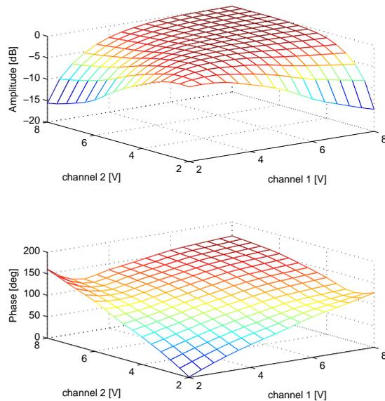
Figure 2: Amplitude and phase modulation with the FVMs.
