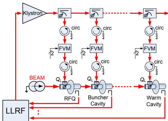
Figure 1: RF control block diagram for HINS.
