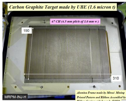
Figure 2: SEEM using carbon-graphite ribbons.
