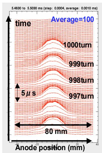
Figure 3: Measured vertical beam profile.
