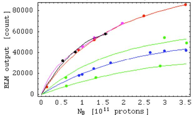
Figure 1: BLM output as a function of the number of lost protons. Green: Arc, blue: slow extraction, red: MR collimator, magenta: fast extraction, black: injection beam dump. At the BLM gain of ~2300 (HV = -1.6 kV).
