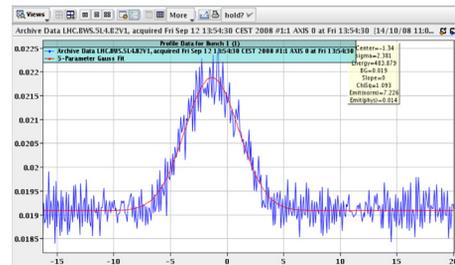
Figure 6: BWS, vertical scan of a circulating pilot bunch.
