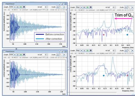
Figure 4: BBQ, first tune measurement and correction.
