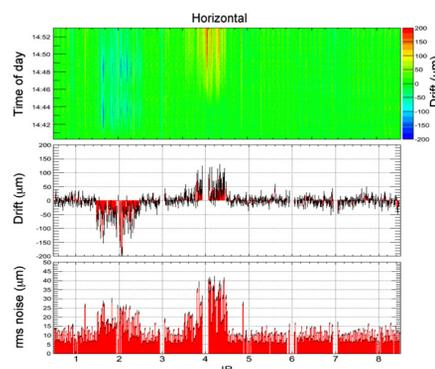
Figure 1: BPM orbit stability in high sensitivity mode.
