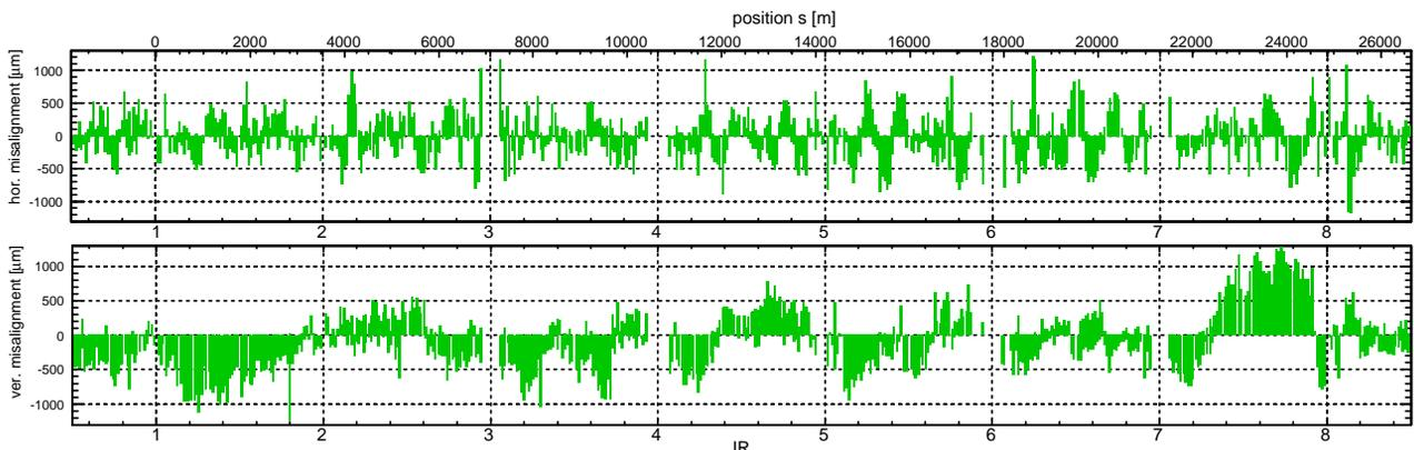
Figure 2: Horizontal and vertical magnet position deviation.
