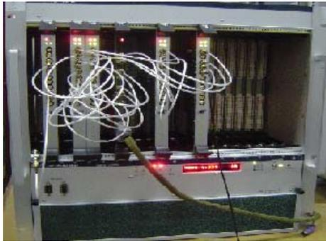
Figure 6: The VME frame timing trigger system.
