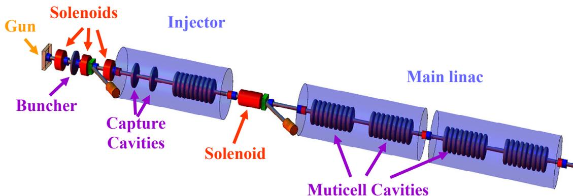
Figure 1: E-linac schematic layout.
