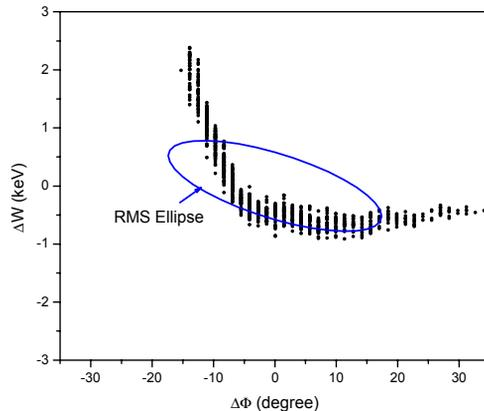
Figure 2: Particle distribution in the  $\Delta\Phi$   $\Delta W$  space at the gun exit. The ellipse is calculated from the longitudinal rms emittance.
