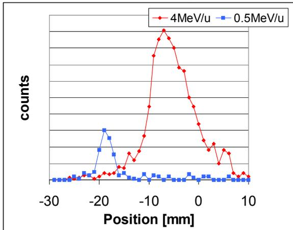
Figure 3: Signal on the diamond detector. The beam components with 0.5 MeV/u and 4 MeV/u are displayed in blue and red. The spatial separation is due to a magnetic dipole field in front of the detector.
