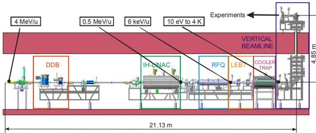
Figure 2: Overview of the HITRAP facility with the major components indicated. DDB – Double Drift Buncher for bunching the beam to adapt it to the longitudinal acceptance of the decelerator, IH – LINAC – interdigital H-type structure for deceleration, RFQ – radio-frequency quadrupole accelerator structure for deceleration, LEBT – Low energy beam transport line for efficient injection into the trap, COOLER TRAP – Penning trap for final deceleration and cooling.
