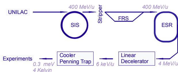
Figure 1: Schematic view on the production of slow, highly-charged ions with HITRAP.
