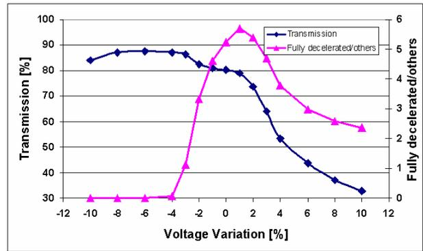
Figure 4: Calculations on the deceleration and transmission of the IH structure using LORASR. Shown is the transmission in blue and the ratio of transmitted particles to decelerated particles in pink versus the variation of the RF amplitude change in percent in the IH tank.
