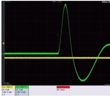
Figure 7: The injection septum voltage waveform.
