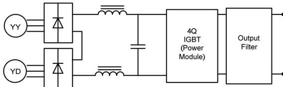
Figure 4: QF/QD Power Converter layout.
