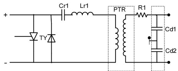
Figure 6: Simplified Injection Septum PS layout.
