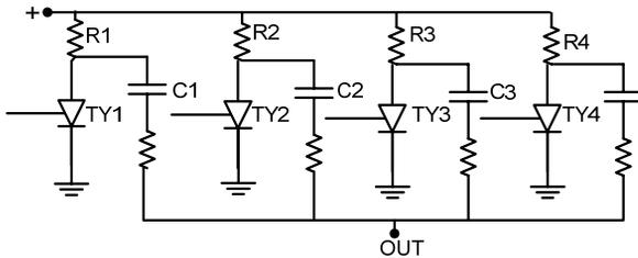
Figure 8: Simplified Injection kicker PS layout.
