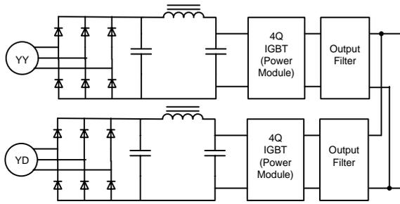
Figure 3: Simplified layout of 2 out of 6 modules for dipole magnet power converter.
