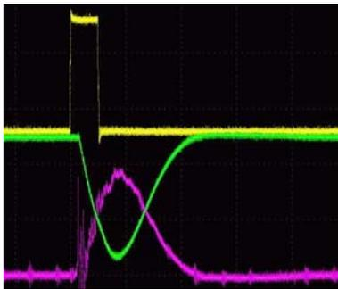
Figure 9: The injection kicker current (Green) measurement results. H:V /div.(100A:2us).
