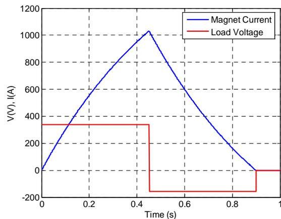
Figure 2: Current/Voltage waveform for the dipole magnet family.
