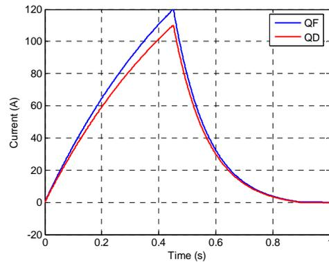
Figure 5: QF/QD typical current waveform.
