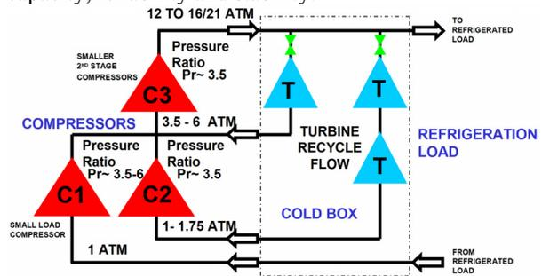
Figure 7: Simplified ganni helium process cycle.
