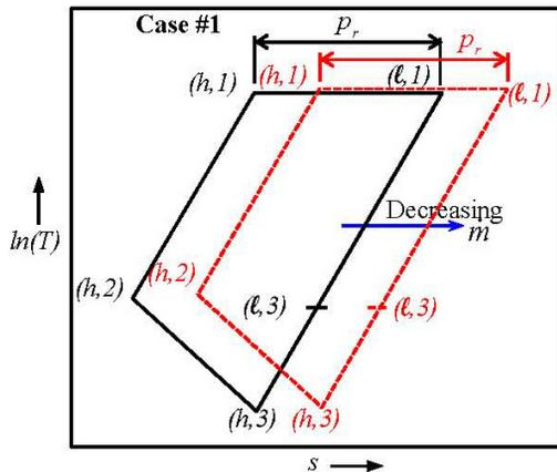
Figure 5: TS diagram of floating pressure process.
