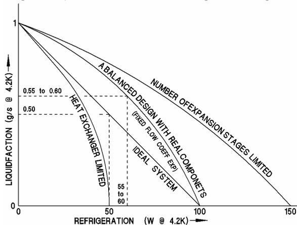
Figure 3: Effect of components on system load capacity.
