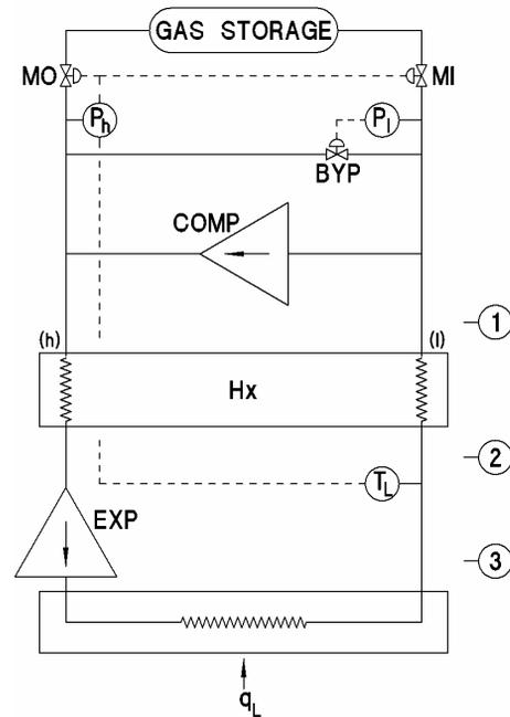
Figure 4: General arrangement for floating pressure process cycle (*patent pending*).
