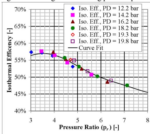
Figure 6: Typical 2<sup>nd</sup> stage screw compressor isothermal efficiency.
