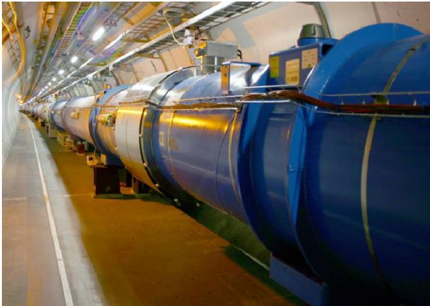
Figure 1: Picture of an LHC arc showing the magnet cryostat envelopes.
