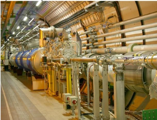
Figure 2: Picture of a long straight section showing a standalone cryomagnet (left) and the QRL line (right).
