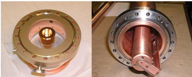
Figure 5: SNS Ceramic RF window (left) and loop RF coupler for MuCool prototype cavity.
