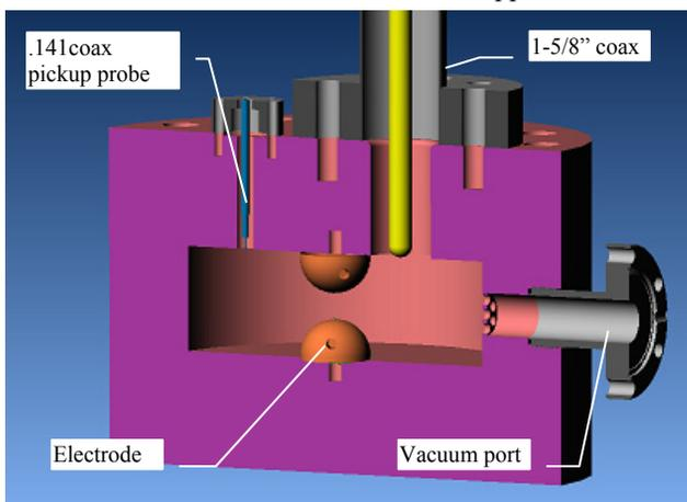
Figure 2: Cutaway view of the 1.3 GHz Cavity
