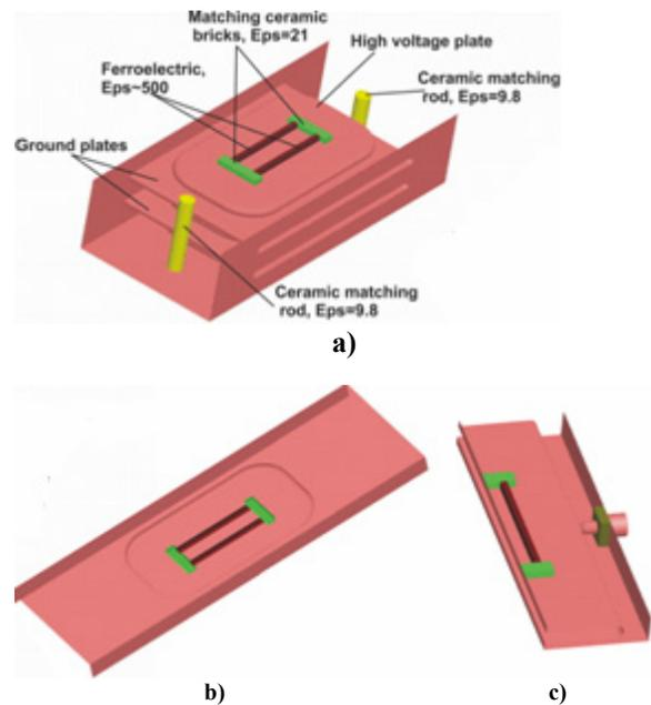
Figure 1: (a) Full geometry of phase shifter. (b) one-third section of phase shifter. (c) HV input.
