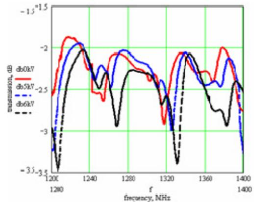
Figure 7: Same as Fig. 6, except in an arrangement where the top wall was resting (under 200 - 400 lbs load) on the ceramic bars and was not bolted to the side walls. Here, the transmission did not drop so much as in Fig. 6, or in some cases even increased. However, in general the transmission level was lower because of leakage radiation through the gaps formed between unbolted walls.
