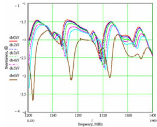
Figure 6: Transmission (dB) vs frequency (MHz). Transmission drops as voltage is increased in the versions with fixed structure height (the top and bottom walls are tethered by the side walls), suggesting a possible piezoelectric contraction of the bars.
