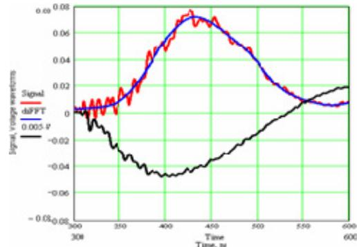
Figure 5: Time-response of the phase shifter.
