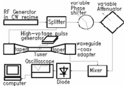
Figure 4: Setup for phase switch speed measurement.
