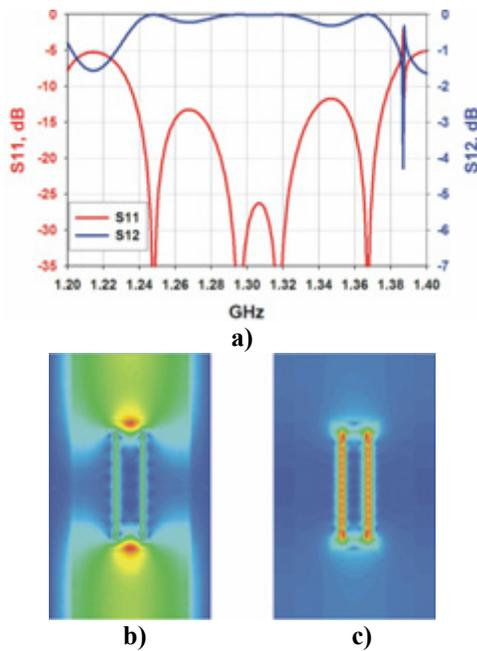
Figure 2: (a) Frequency response for one-third section. (b) Electric field. (c) Magnetic field.
