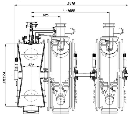
Figure 1: Schematic view of three bi-metal accelerating cavities.
