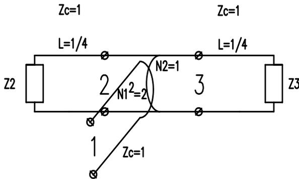
Figure 3: Equivalent circuit of double waveguide to coaxial transition: 1 – waveguide port, 2 and 3 – coaxial line ports,  $Z_c$  – normalized characteristic impedance,  $Z_2$  and  $Z_3$  – cavity input impedances.
