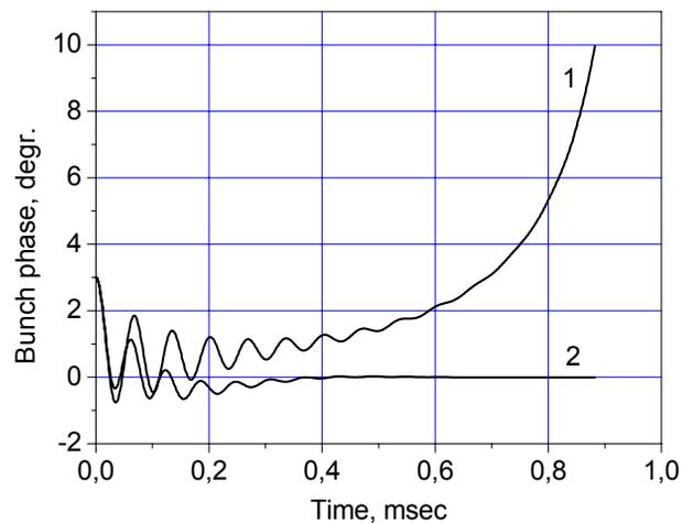
Figure 4: Bunch phase motion: 1 – without feedback, 2 – with feedback.
