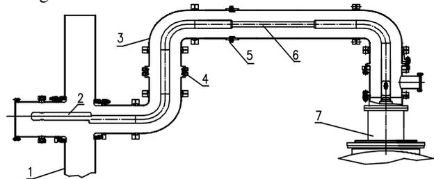
Figure 2: Schematic drawing of the coaxial line with waveguide to coaxial transition: 1 – waveguide, 2 – antenna of the waveguide to coaxial transition, 3 – 75 Ohm coaxial line, 4 – directional coupler, 5 – RF probe, 6 – matching 100 Ohm transformer, 7 – accelerating cavity.
