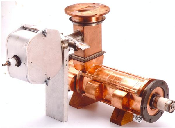
Figure 1: 6 MeV linac tube.
