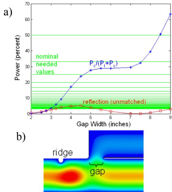
Figure 2: a) Coupling ratio as a function of gap length and the reflection amplitude to be matched by a ridge; b) Half cross-section with electric field plot for a 7.9375 cm gap, tapping off about 6.6% or 1/15 of the power.
