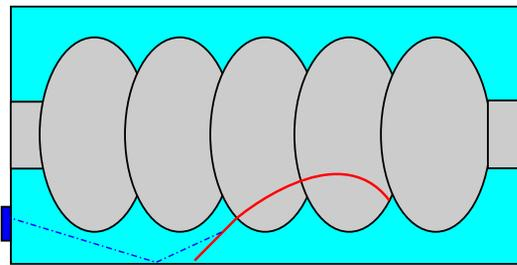
Figure 2: Sketch of the basic concept. An electron emitted from the surface gets accelerated and goes through the cavity wall. It emits a Cerenkov photon which gets reflected from the inner surface of the helium vessel into the optical port where it can be seen by a photodetector.
