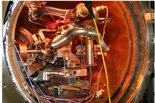
Figure 1: Typical layout showing an rf cavity (in the center) buried inside layers of heat shield and rf and cryo plumbing in a cryostat (from the Fermilab ILCTA-MDB Horizontal Test Stand). X-ray detectors are outside the cryostat.
