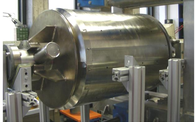
Figure 4: The shield around the cavity.
