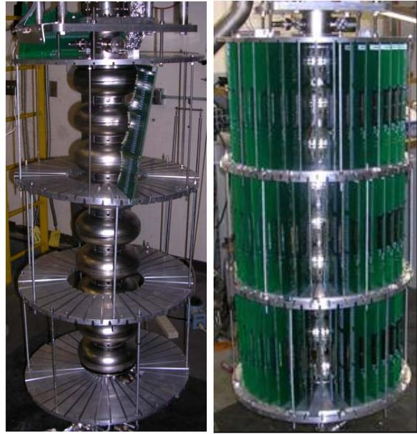
Figure 1: A 1.3 GHz, 9-cell cavity with T-mapping boards supporting plates (left) and full assembly of boards around the cavity (right).
