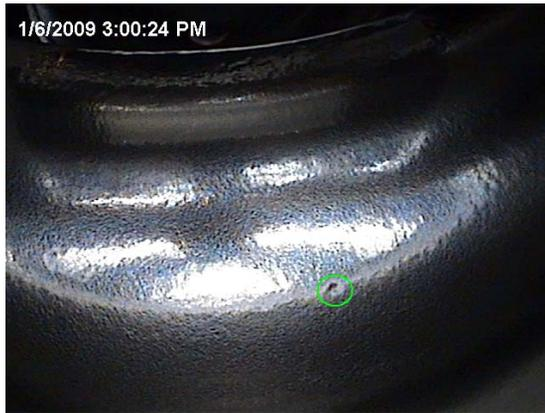
Figure 6: A defect found on a stiffening ring welding area in cell 2 at  $30^\circ$  that seems responsible for FE in  $\pi$  mode.
