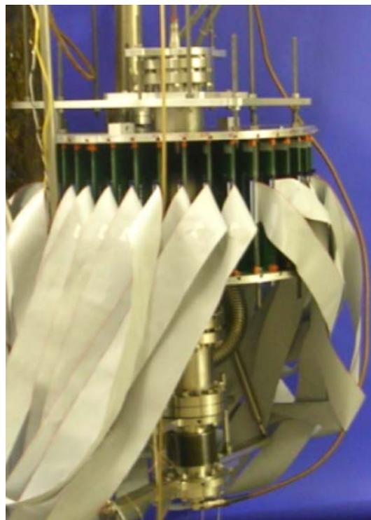
Figure 4: The 805 MHz single-cell cavity surrounded by temperature mapping boards.
