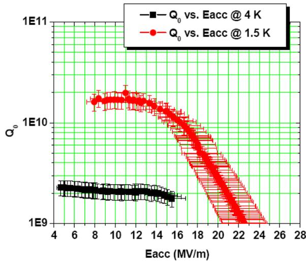
Figure 5:  $Q_0$ - $E_{acc}$  curve of the 805 MHz single cell cavity.
