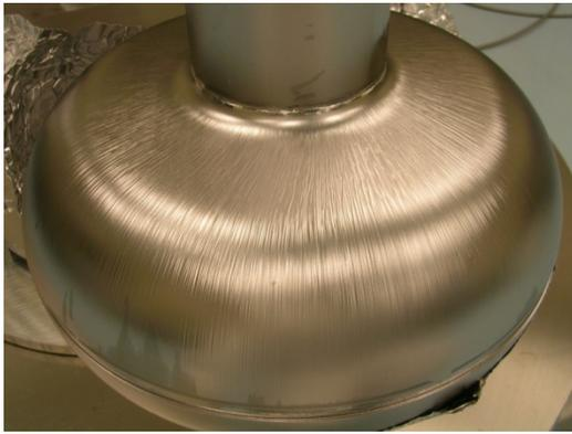
Figure 1: Outside surface after BCP of 150  $\mu\text{m}$ . This side was facing downward when BCP was done. Traces of bubbles are clearly seen. The surface facing upward was smooth.
