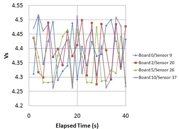
Figure 8: T-map noise level of 4 sensors measured at 4 K. The horizontal axis corresponds to the data number. The data taking time per sector is 2 s.
