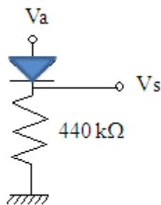
Figure 6: Diode test circuit.
