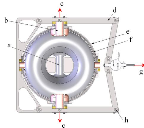
Figure 3: Section view of the tuner at the mid plane of the cavity: (a) drift tube; (b) beam tube; (c) resulting cavity; deformation force; (e) helium vessel; (f) outer conductor; (g) applied tuning force; (h) compliant pivot.
