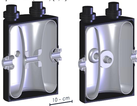
Figure 1: CAD representation of the beta 0.53 half wave.
