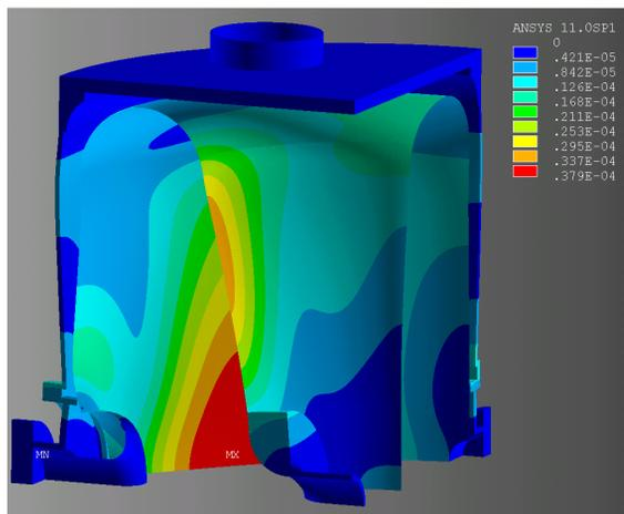
Figure 2: Displacement contours from the mechanical model in ANSYS.
