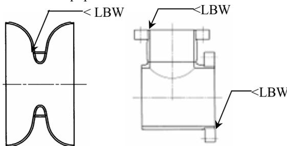
Figure 7: The procedure for joining the stiffener and half-cell by LBW for ILC proposal.
