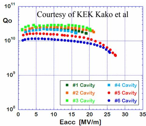
Figure 2: Q-E curve at the first vertical test of the STF 1.5A-type cavities (#5, #6) compared with STF 1.0-type cavities (#1-#4) by KEK.
