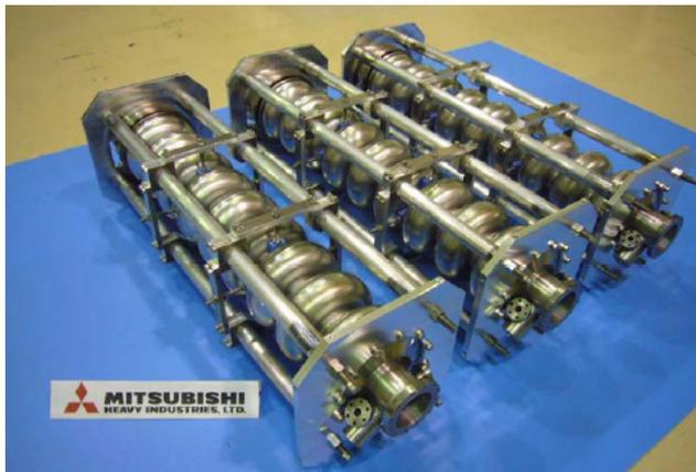
Figure 1: The STF 1.5B-type cavities (#7-#9) fabricated at MHI in March 2009.
