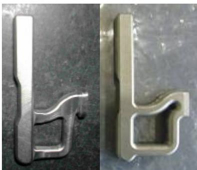
Figure 3: The inner conductor of the HOM coupler for STF1.5A (left) and STF1.5B (right).
