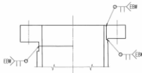
Figure 6: The NbTi flange for STF1.5A (left) and STF1.5B (right).
