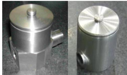
Figure 4: The outer conductor of the HOM coupler for STF1.5A (left) and STF1.5B (right).
