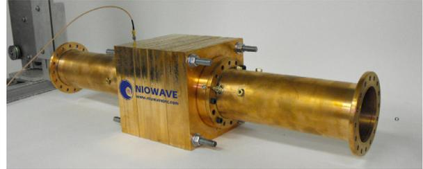
Figure 6: Copper prototype undergoing bead perturbation field measurements.
