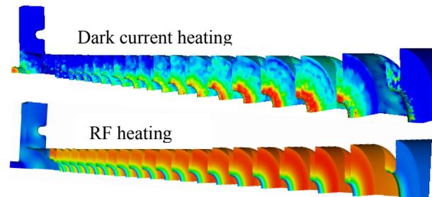
Figure 4: Top: dark current heating distribution. Bottom: RF heating distribution for comparison.
