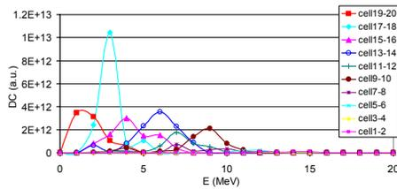
Figure 5: Dark current amplitude and energy v.s. emission location at 97 MV/m gradient. Cell 19-20 are the cells at the output end.
