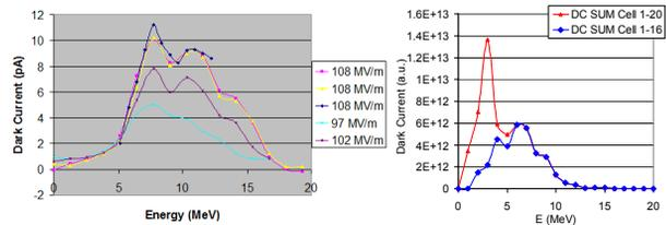
Figure 8: Dark current spectrum. Left) measured; Right) simulation – red includes all cells, blue has a similar shape as measurement but includes cells 1-14 only.
