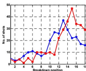
Figure 7: Breakdown rate significantly higher at the output end (Red real cell timing, blue linear cell timing).
