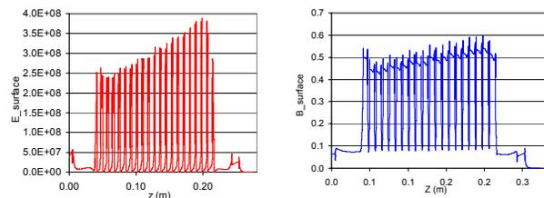
Figure 2: The accelerating field profile along the structure obtained from S3P simulation.
