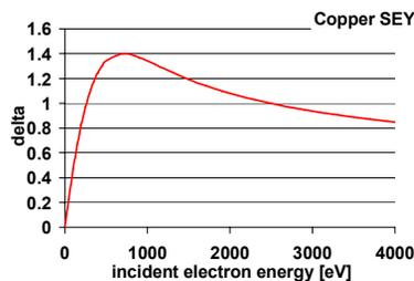
Figure 3: SEY distribution for copper. The SEY peaks at around 800 eV.
