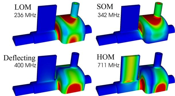
Figure 6: The LOM and SOM are damped by the combined coaxial coupler; the HOM is damped by the waveguide coupler; and the operating mode is not affected by these couplers.
