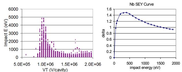
Figure 3: Left: impact energies of resonant trajectories versus deflecting voltage; Right: typical SEY distribution for Niobium. The SEY peaks at around 200-400 eV.
