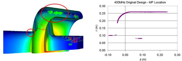
Figure 2: Distribution of resonant trajectories.
