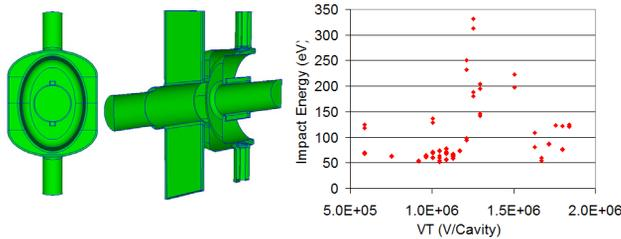
Figure 4: Left: optimized cavity shape that eliminates the multipacting trajectories; Right: impact energy of resonant trajectories as a function of deflecting voltage.
