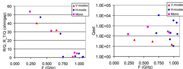
Figure 5: The shunt impedance R/Q and damping results for the LOM, SOM, and HOM modes.
