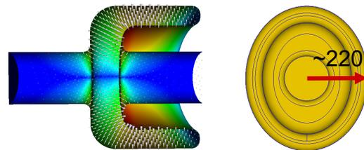
Figure 1: Cell profile of the half wave resonator 400MHz crab cavity. Left: cavity z-y cross section, the arrows show the mode pattern of the electric field; Right: cavity x-y cross section shown the squashed shape to split the degeneracy of the x and y polarized dipole modes.
