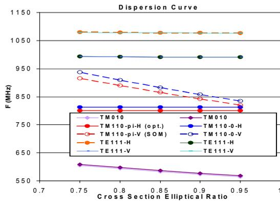
Figure 5: Dispersion curve for the 2-cell crab cavity as a function of the cell squash ratio. The beampipe cutoff frequency is 1.2GHz.
