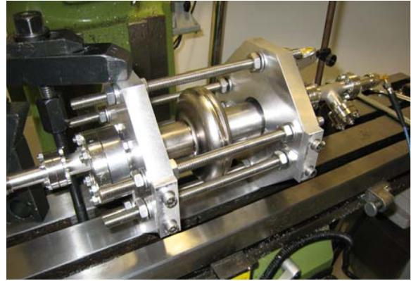
Figure 2: Cavity in its tuning jig.
