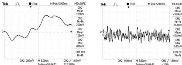
Figure 7: Phase jitter between C1 and C3 (unlocked, left, and locked, right), 1mV = 20 millidegree phase difference.
