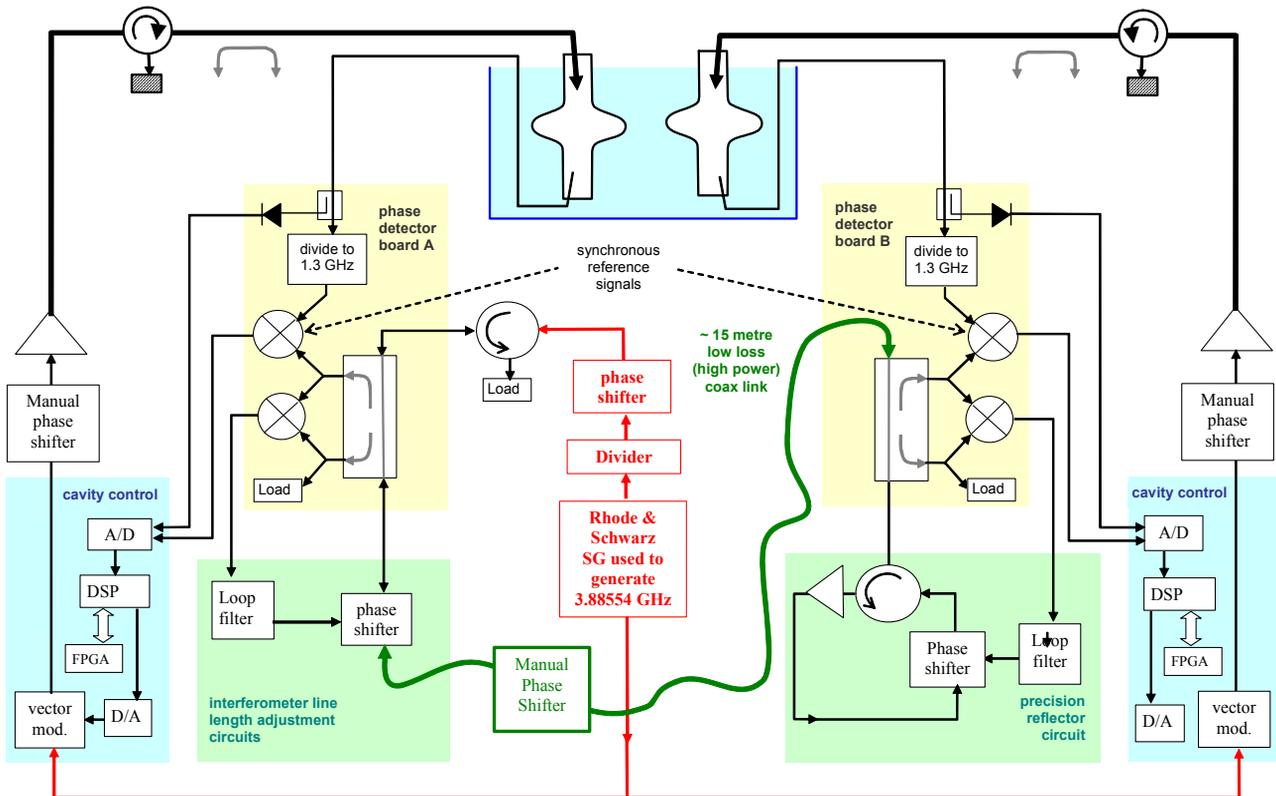
Figure 6: Schematic of the phase control system used for the vertical tests.
