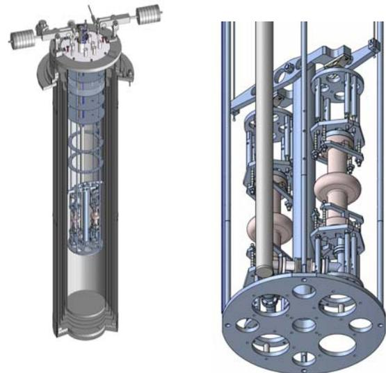
Figure 3: View of the cells in the cryostat and detail of the cavities, tuner arms and load-cells.
