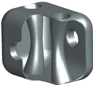
Figure 1: Concept of a TEM deflecting structure with curved resonant bars and variable cross-section [2].
