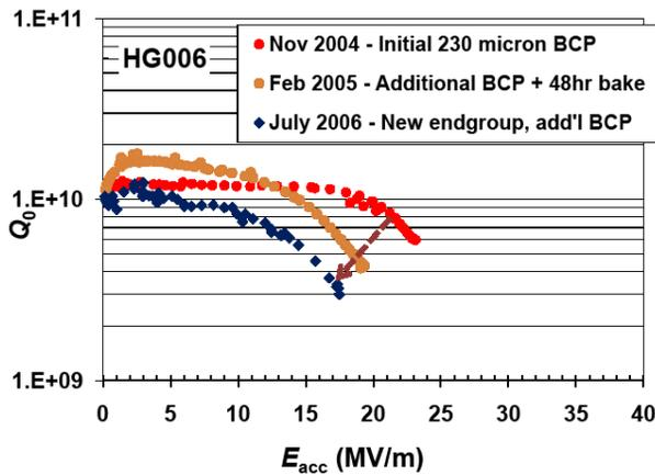
Figure 2: Sequence of degrading performance of cavity HG006 with incremental BCP cycles.
