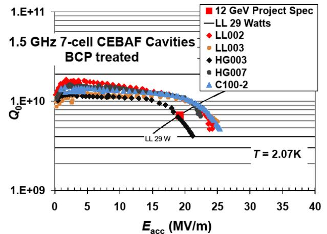
Figure 1: Characteristic Q-drop of fine-grain niobium cavities with JLab BCP etch preparation 2004-2007.
