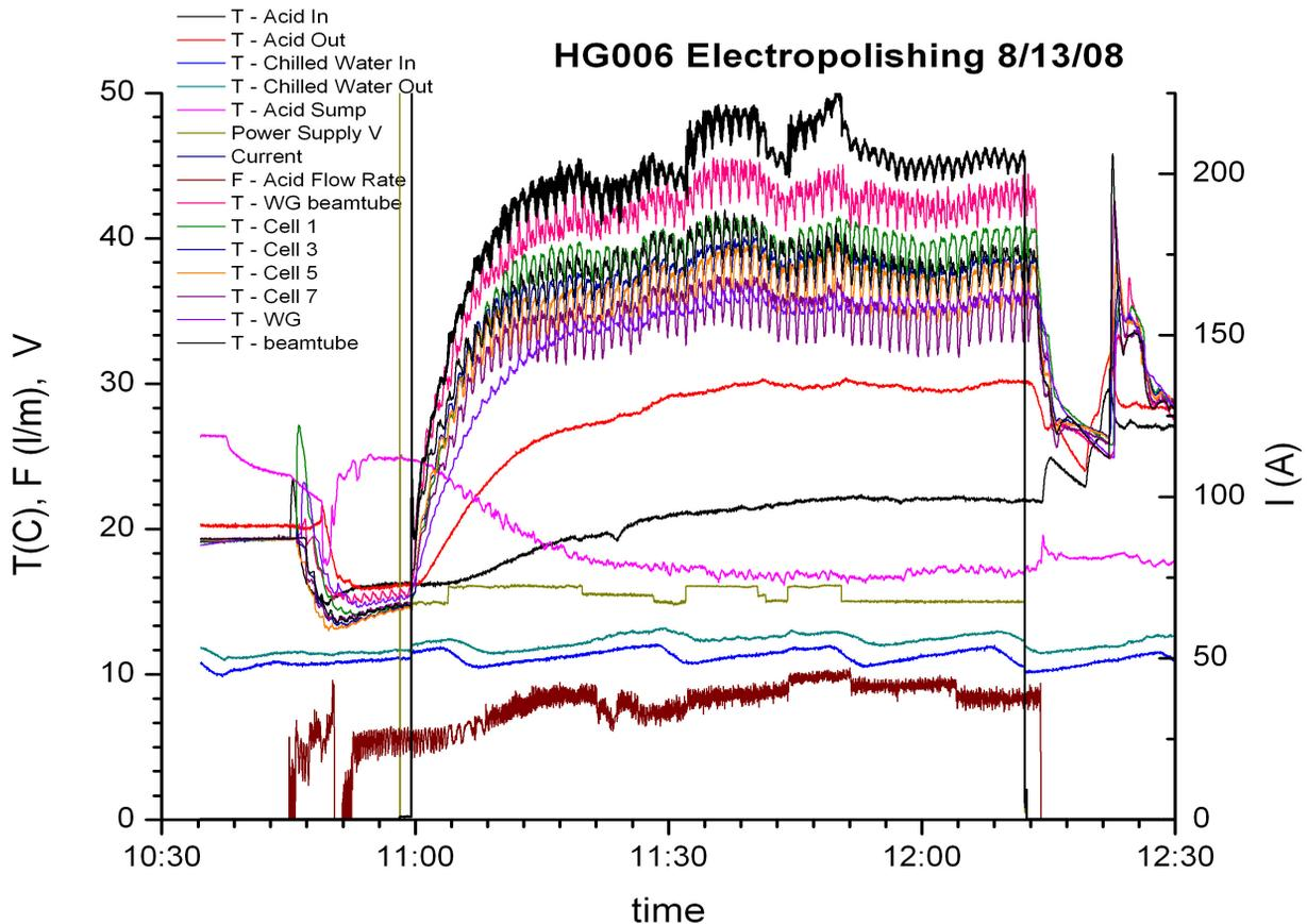
Figure 4: Electropolishing process parameters for removal of 30 microns from the JLab 7-cell cavity HG006.
