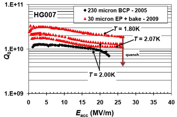
Figure 6: HG007 rf test data before and after EP.
