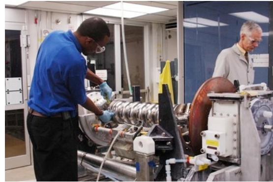
Figure 3: 1.5 GHz 7-cell cavity HG006 being assembled into the JLab horizontal electropolish machine.
