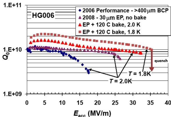
Figure 5: Performance of HG006 with initial light electropolishing treatment.
