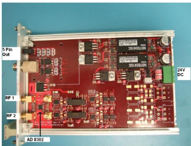
Figure 3: Final circuit board.
