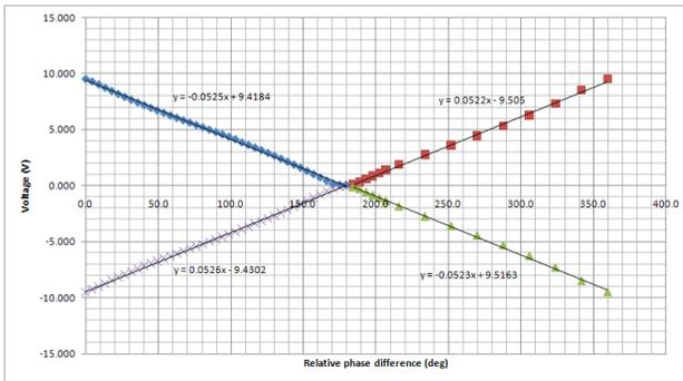
Figure 6: Phase response curve.
