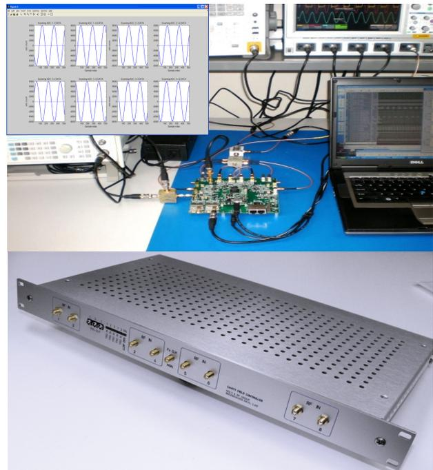
Figure 6: The first prototype of the cavity field controller hardware currently under tests for its I/O functions and SNR characterization.
