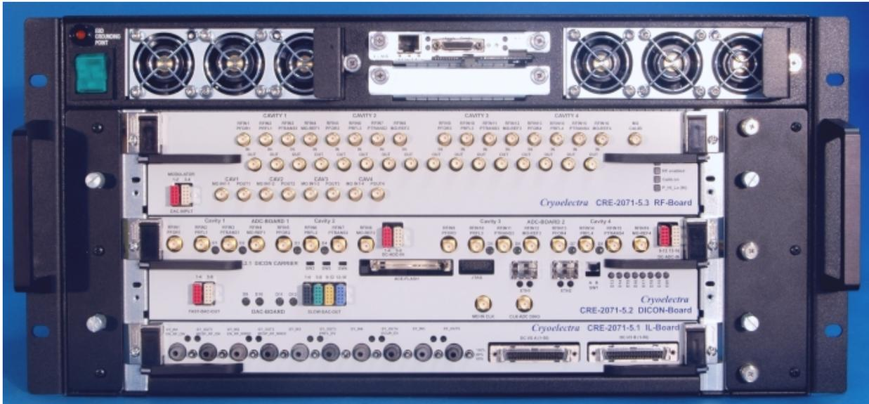
Figure 4: LLRF subsystems integrated in a standard ATCA crate. ATCA modules: (Top) 16 channel RF-module with 4 channel Modulator daughter board, (Middle) DICON-Module with two 8(+8)-channel ADC-boards, Clock-Multiplier-Board and 8(+16) channel DAC-Board. (Bottom) Interlock-Module with 5 optical inputs and 5 outputs.
