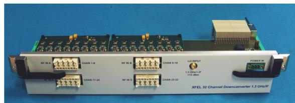
Figure 2: 32 channel ATCA Rear Transition Module (RTM) carrying four 8 channel down converters as daughter boards.
