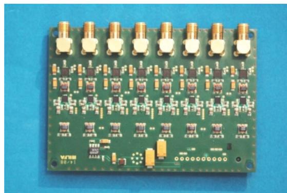
Figure 1: 8 channel down converter daughter board for conversion of 1.3 GHz to 50 MHz.
