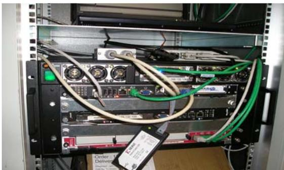
Figure 3: Set-up used for the first demonstration with DACs (in-house design), and downconverters on the rear transition module. The block diagram of hardware is presented in figure 2. All required signals: external source
