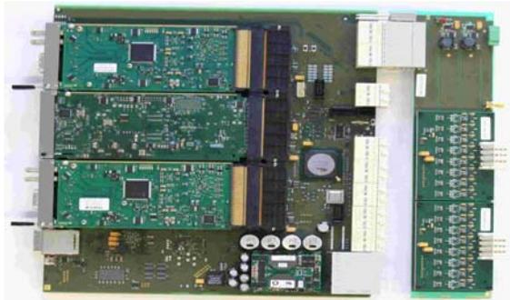
Figure 5: ATCA LLRF system consisting of ATCA carrier, AMCs and RTM module with downconverters.
