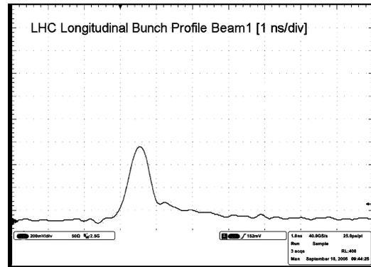
Figure 1: First Longitudinal bunch profile of Beam 1 acquired from the APWL wall-current monitor. 1 ns/div.
