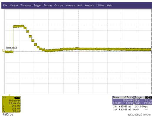
Figure 4: Bunch-RF phase at injection in the presence of an injection phase error and with phase loop ON. 500 μs/div.
