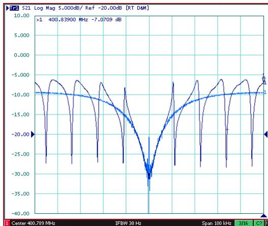
Fig. 3: Effective cavity impedance, 100 kHz span around the cavity centre frequency of 400.789 MHz.
