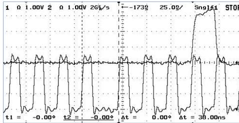
Fig. 6: Read data of RAM are synchronized to the read clock (bottom) changing just before the end cycle (top).
