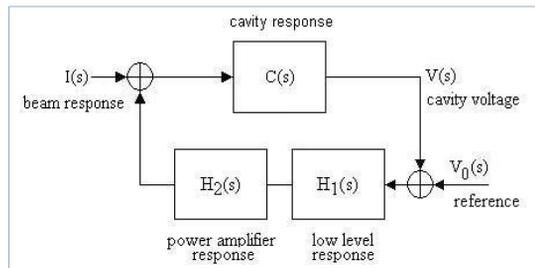
Fig. 1: Closed loop response for a cavity feedback system.
