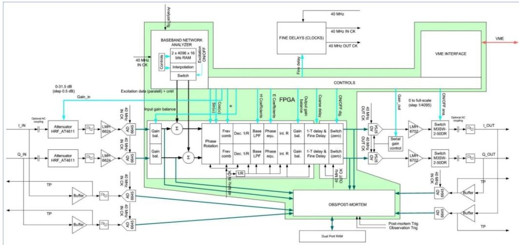
Fig. 2: The LHC 1-Turn Feedback implemented in the module EDA-01150. The shaded area denotes the FPGA.
