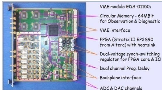
Fig. 7: LHC 1-T Feedback, VME module EDA-01150.
