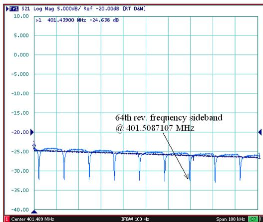
Fig. 4: Effective cavity impedance, 100 kHz span around the frequency of 401.489 MHz.
