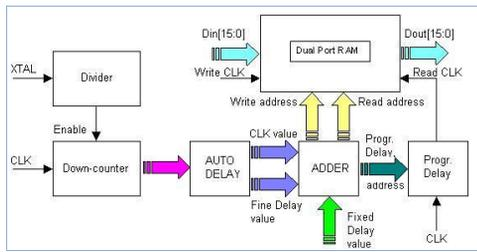
Fig. 5: Automatic Delay Compensation. Block diagram.
