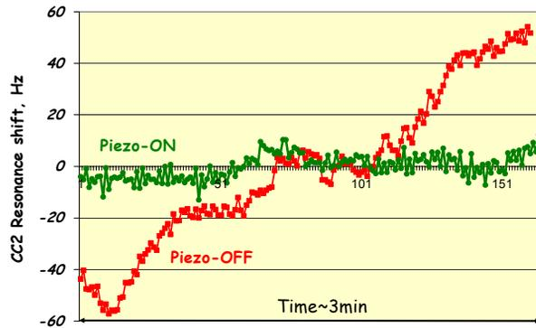
Figure 4: Resonance stability of CCII at 4K.
