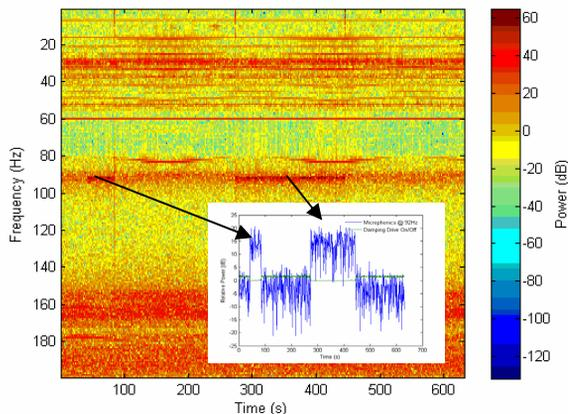
Figure 5: Active damping of externally induced vibrations.
