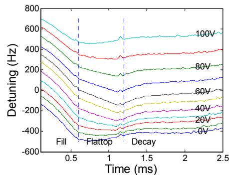
Figure 1: Instantaneous detuning of the cavity during the RF pulse as a function of piezo bias voltage.
