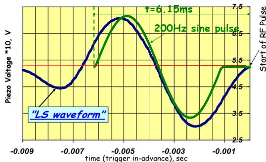
Figure 2: A comparison of LFD compensation pulses.
