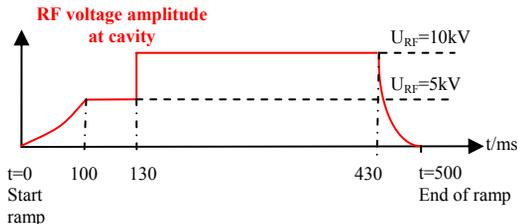
Figure 3: Voltage ramp at the acceleration cavity for the excitation of quadrupole oscillations in the synchrotron SIS12/18.
