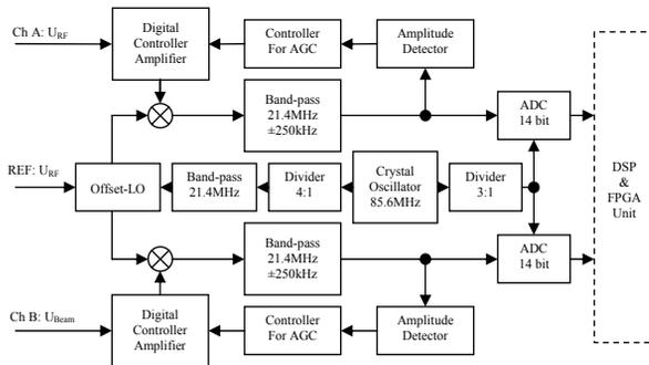
Figure 1: Hardware architecture of the analogue signal processing.
