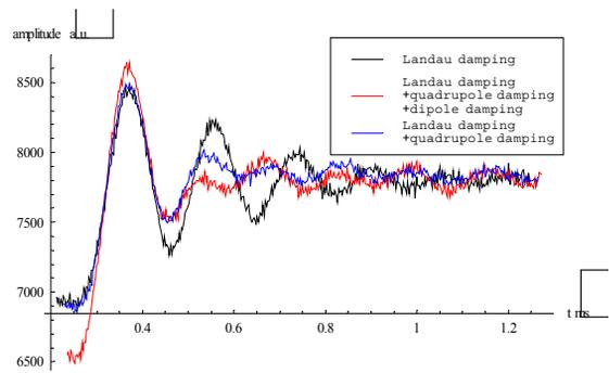
Figure 4: Measured averaged amplitude data of the DSP acquisition system in time domain. Displayed are the first 1.1ms after the voltage amplitude jump. In the caption it is shown which colour represents which damping system state.
