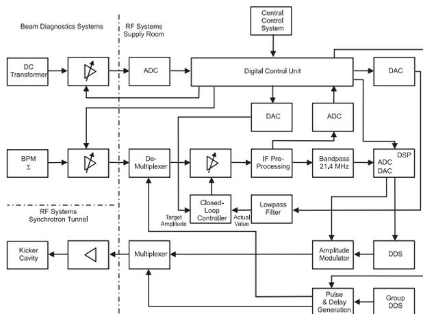
Figure 6: Block diagram of the overall signal processing planned for SIS100. (DAC: digital-to-analogue converter).
