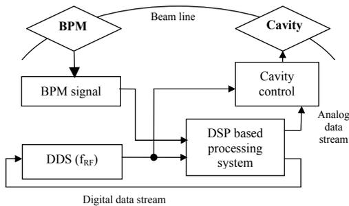
Figure 2: Simplified setup of the data acquisition using the DSP based processing system in the closed loop damping setup for dipole and quadrupole oscillation modes in SIS12/18. (DDS: direct digital synthesis).
