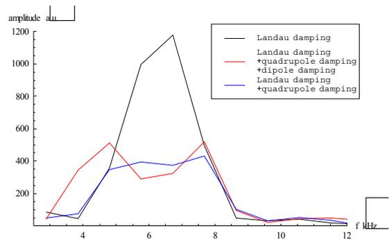
Figure 5: Measured amplitude data of the DSP acquisition system in frequency domain. In the caption it is shown which colour represents which damping system state. To create the spectra the time interval pictured in Fig. 4 has been used (about 1.1ms from voltage jump to the end of the picture).
