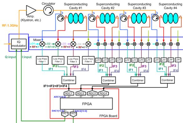
Figure 2: Schematic diagram of system configuration.
