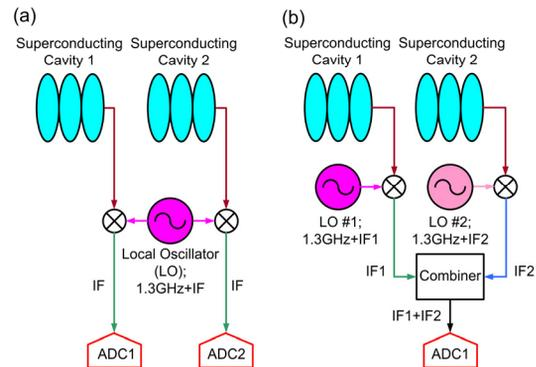
Figure 1: Schematic diagram of the digital LLRF system: (a) Typical system and (b) IF-mixture technique.
