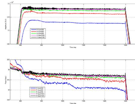
Figure 6: Amplitude and phase at the flat top with different proportional gain.
