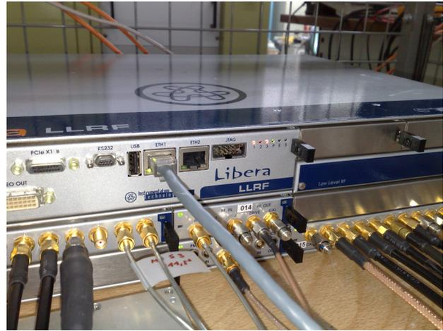
Figure 1: Libera LLRF, an industrial 19" 2U rack-mount chassis digital RF stabilization system, controlling the 1.3 GHz EMMA test set-up with 10 kW.
