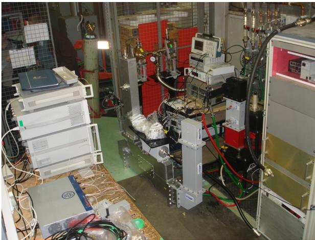
Figure 3: EMMA FFAG test setup. In the background the two copper cavities, the waveguide hybrid distribution system in the middle, the IOT and the HVPS on the right, the Libera LLRF with the MO reference on the left are visible.
