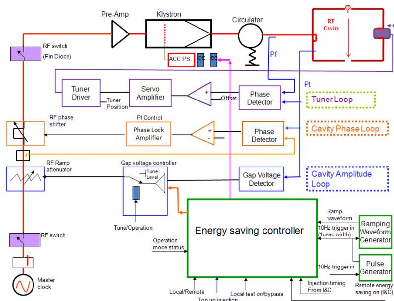
Figure 1: The block diagram of the booster RF system in TLS
