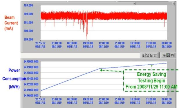
Figure 4: Power consumption reduction effects of the energy saving controller.
