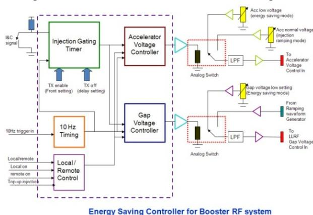
Figure 2: Function blocks of the energy saving controller.
