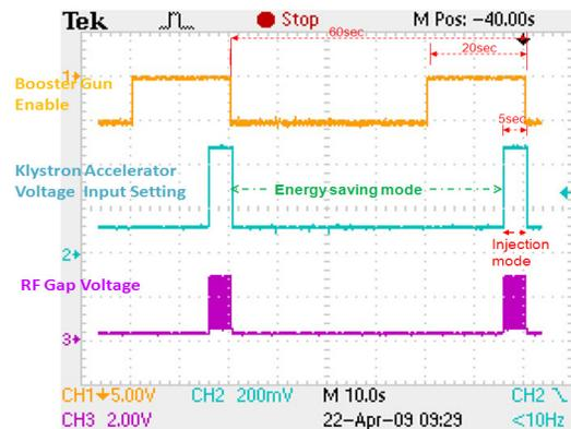
Figure 3: Timing measurement of the energy saving controller.
