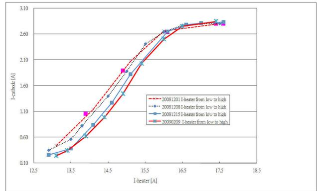
Figure 5: The testing results of the cathode current variation as functions of heater current.
